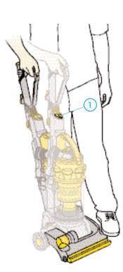
After plugging machine into mains, press on/off button 1, push cleaner head down with foot and pull handle towards you.
